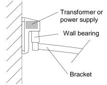
In case of the lights Mach LED 120, Mach LED 120F, Mach 120 and Mach 120F the transformer is positioned in the wall bearing.
